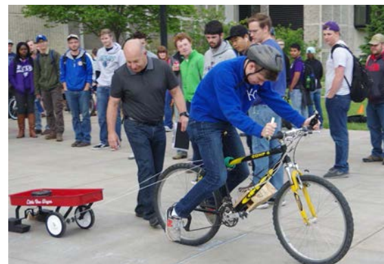
A student balances on his team's vehicle as their cordless drill powers him through the sled pull challenge.
