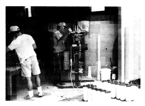
Small laboratory silos (lower right) are a valuable research tool for following silage fermentation dynamics. Here, silage is uniformly packed into the laboratory silos using a hydraulic press.
