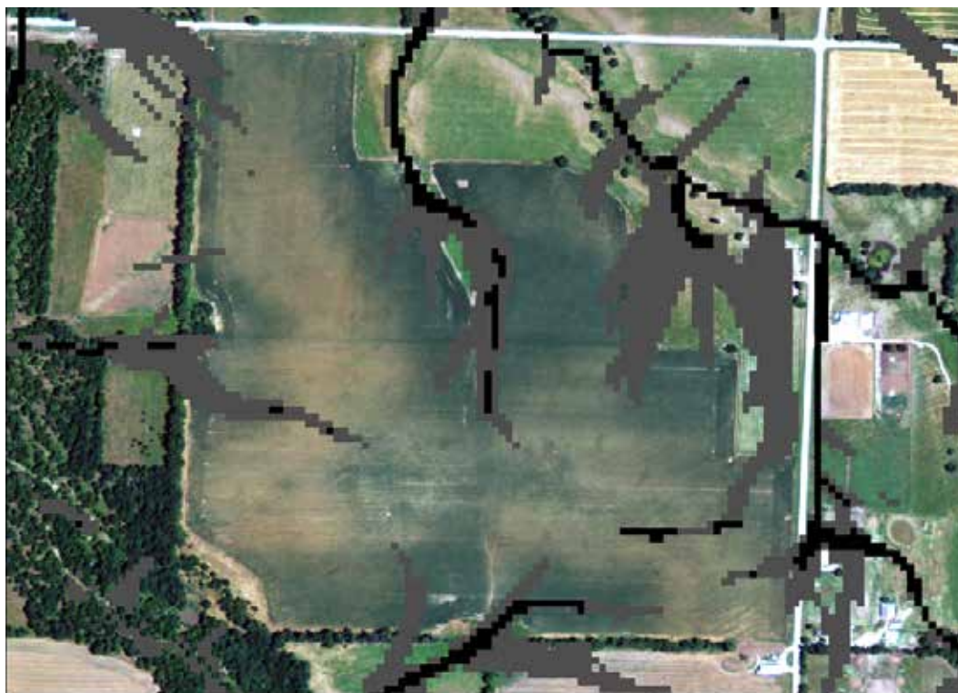
Figure 5. Terrain analysis of the crop field showing areas of high runoff potential.
