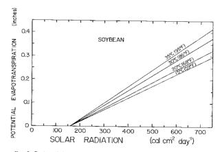
*c*ig. 3. Potential evapotranspiration for soybean as a function of solar radiation and mean temperature.
