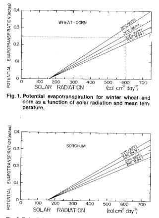
Fig. 2. Potential evapotranspiration for sorghum as a function of solar radiation and mean temperature.
