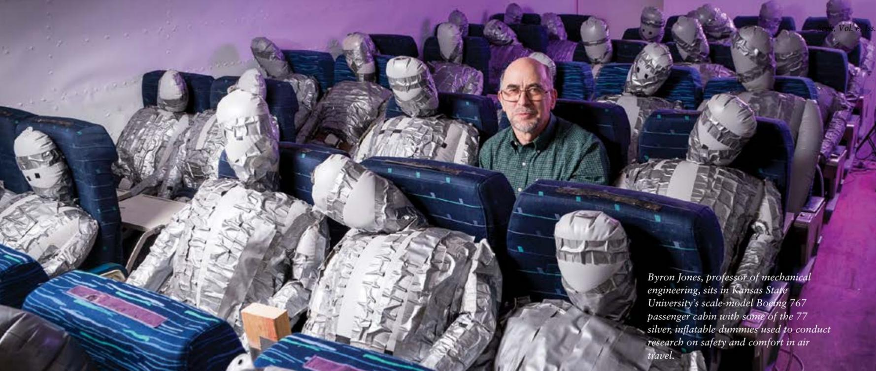
*Byron Jones, professor of mechanical engineering, sits in Kansas State University's scale-model Boeing 767 passenger cabin with some of the 77 silver, inflatable dummies used to conduct research on safety and comfort in air travel.*
