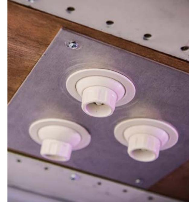
*Air outlets (top) and sensor connectors help researchers with experiments for air cabin comfort.*
