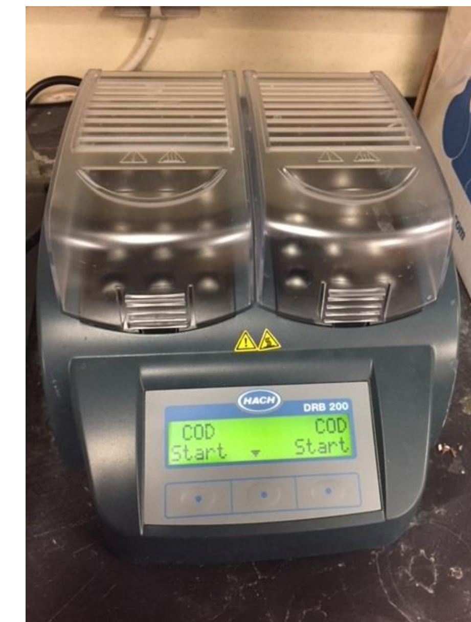
Figure 4. HACH digital reactor block for COD digestion.
