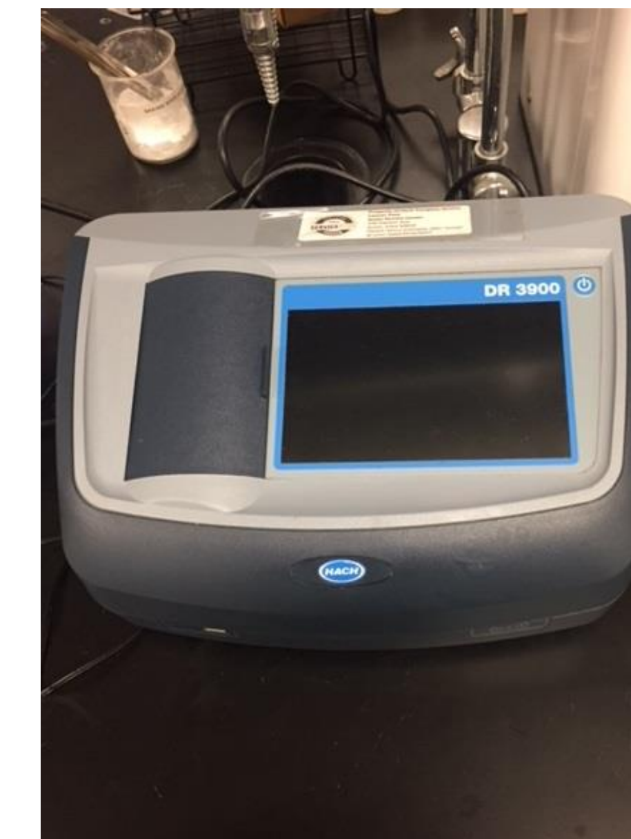
Figure 5. HACH spectrophotometer used for reading COD levels.
