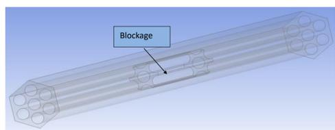
CFD model of geometry with blockage
