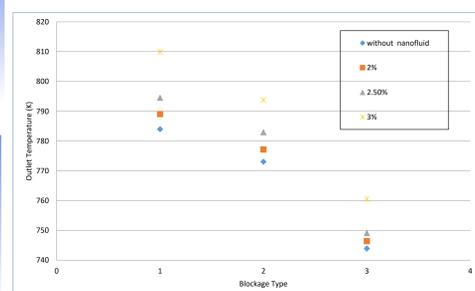
Fig. 2 Bundle outlet temperature for different Nanofluid concentrations
