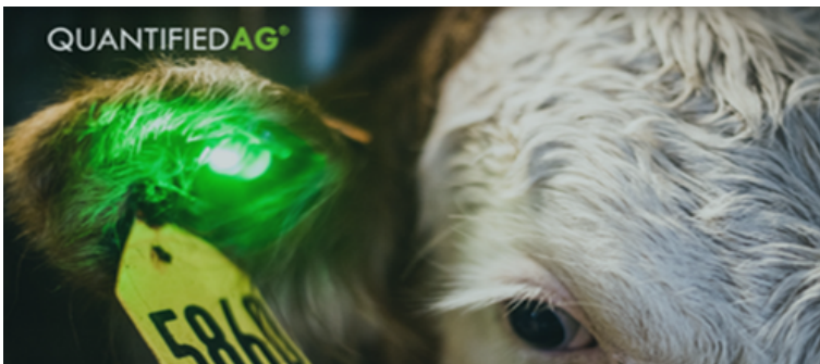
Figure 12-10. QuantifiedAg Tag measures animal temperature and activity level to provide inputs for the producer interface, where a list of sick animals to treat is generated. The indicator light on the tag identifies which animals need treatment.
