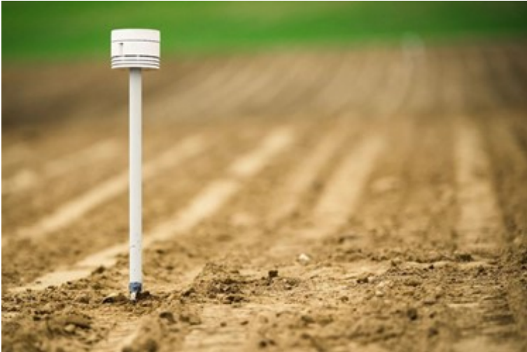
Figure 12-6. OneSoil Agricultural in-ground weather sensor monitors soil moisture and temperature
