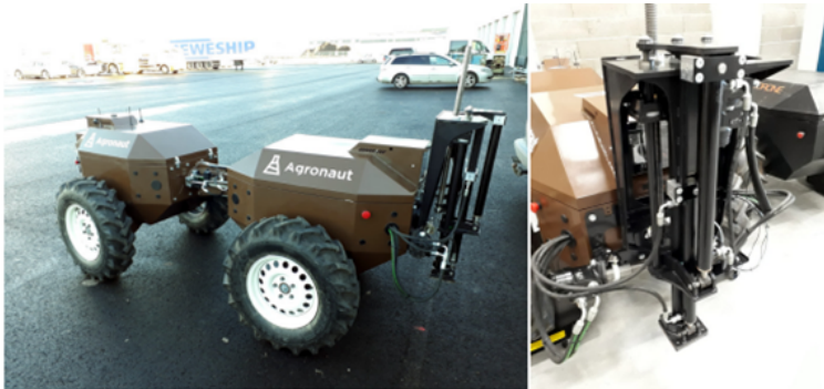
Figure 12-2. Unmanned ground vehicle designed for autonomous soil sample collection by Estonian University of Life Sciences
