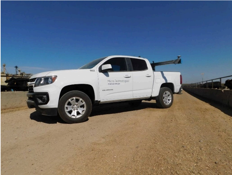
Figure 12-13. Accu-Trac Vision bunk scanner arm for estimating cattle feed remaining from the previous day
