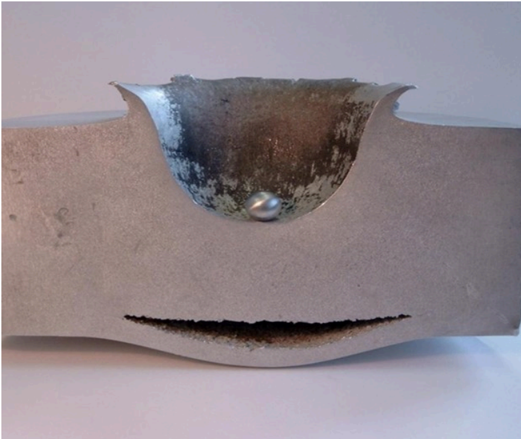
Figure 6-4: Lab Test Result Small Aluminum Ball Hitting Aluminum Block at 7 KM per second (Courtesy Scientific American and ESA)
