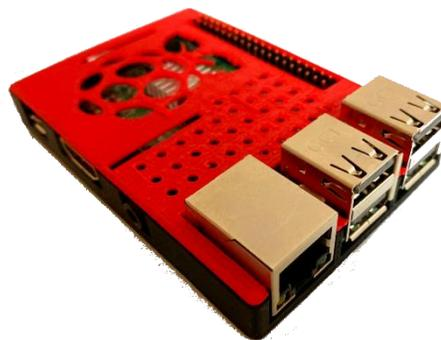
Figure 2: Raspberry Pi with 3D Printed Case
