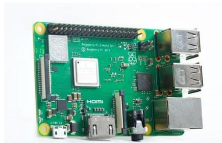
Figure 1: Raspberry Pi 3 Model B+ ([Raspberry Pi Foundation, n.d.-a](#))
