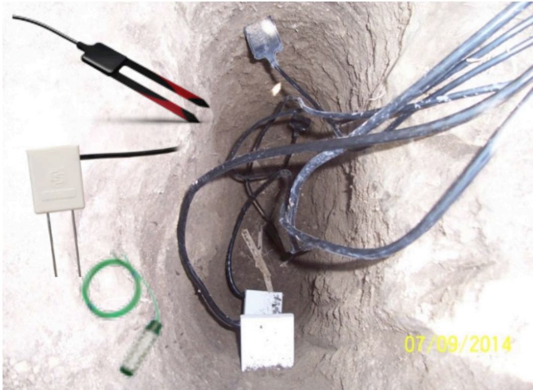
Figure 3. Three different soil moisture sensors (Watermark, CS655, and Decagon 10HS) installed at different depths (1, 2, and 3 feet) were established in the SWREC plot and a farmer's field.
