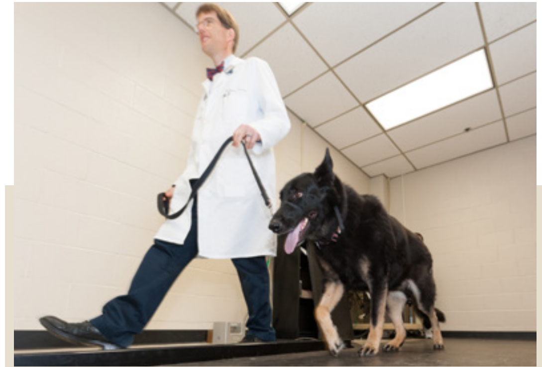
A pressure-sensitive walkway provides objective data of a dog’s pain severity by measuring how much weight the dog puts on each foot — a first in canine stem cell studies.
