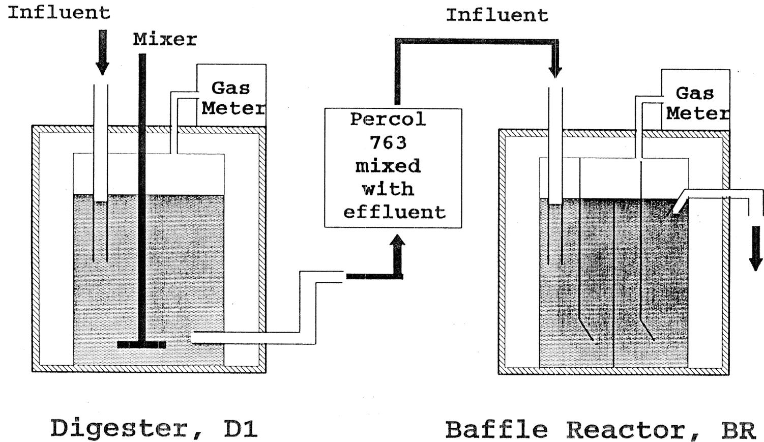
Figure 1. The Digester (D1) - Baffle Reactor (BR) System.
