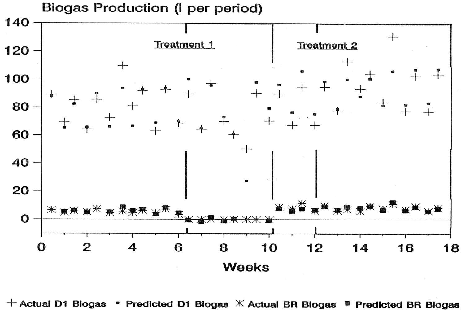
Figure 3. Actual and predicted digester 1 and baffle reactor gas production values over weeks.
