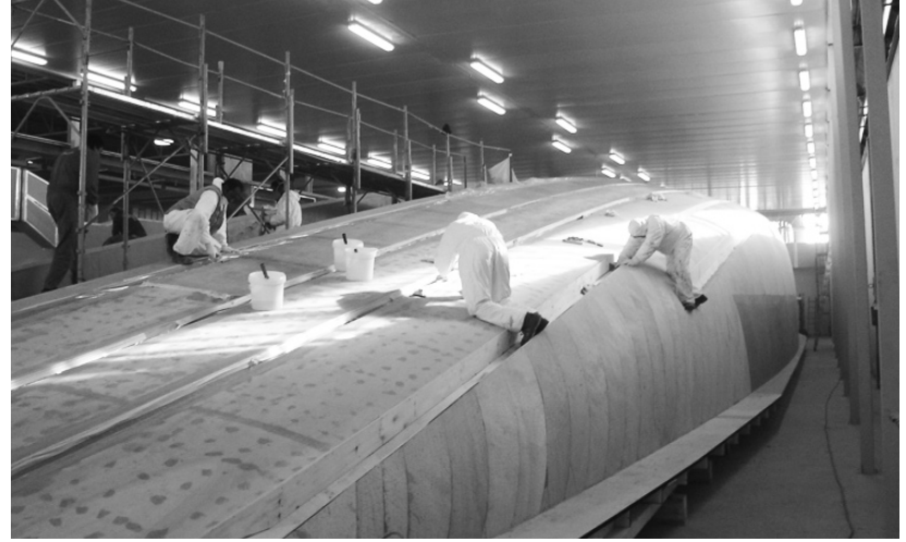
Manual lay-up of carbon fiber yacht hull
