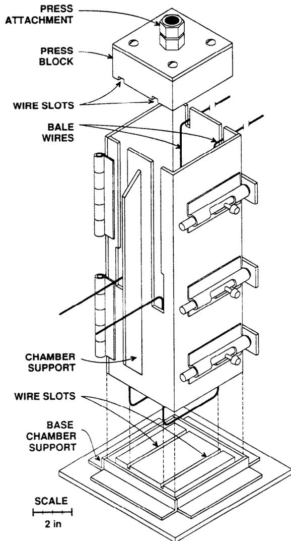
**Figure 1. Scaled Drawing of the Laboratory Baling System**
