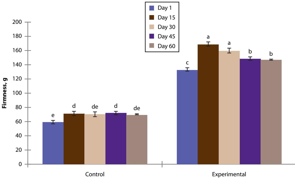
**Figure 2. Yogurt firmness during 60 days of storage. Control: nonfat dry milk (NDM) (12.5%) processed at 90°C for 7 minutes. Experimental: NDM (10%) + whey protein isolate (2.5%) processed at 70°C for 20 minutes.**
