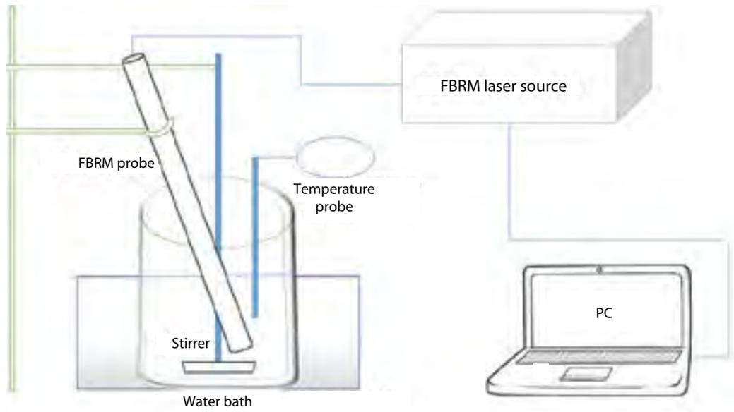
Figure 2. Experimental setup for evaluation of lactose crystallization using focused beam reflectance measurement (FBRM).
