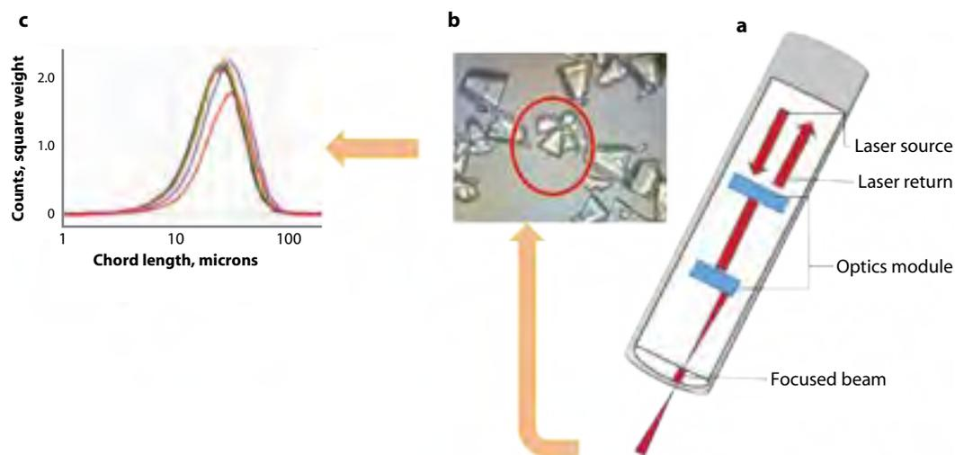
**Figure 1. (a) Focused beam reflectance measurement (FBRM) probe design, (b) detection of particles by probe using a laser moving at constant velocity, and (c) chord length distribution graph obtained from crystal distribution.**
