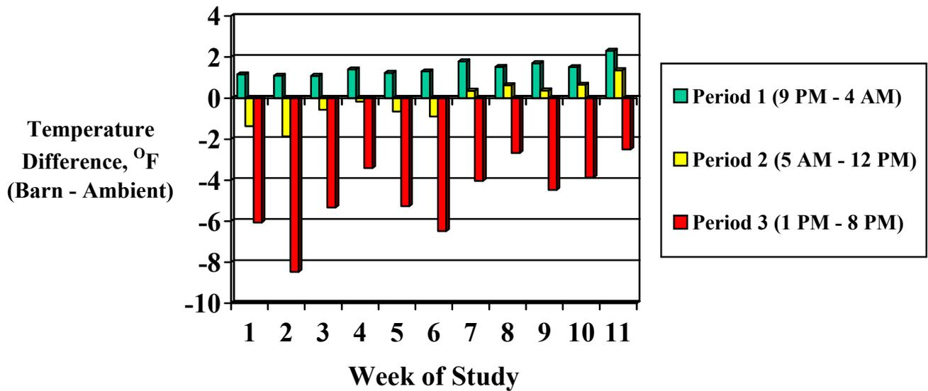
Figure 5. Effect of Evaporative Cooling on Temperature Difference (barn-ambient) during Three Different Periods of the Day in Tie Stall Barns during the Summer of 2001.
