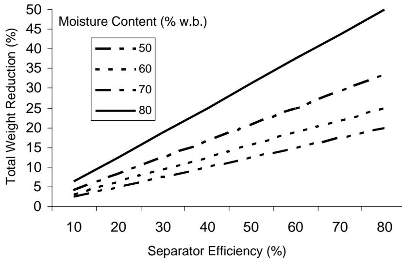
**Figure 2. Impact of Solid Separator Efficiency and Final Moisture Content of the Separated Material on the Volume Reduction Assuming a Cow Excretes 140 lb of Manure per Day.**
