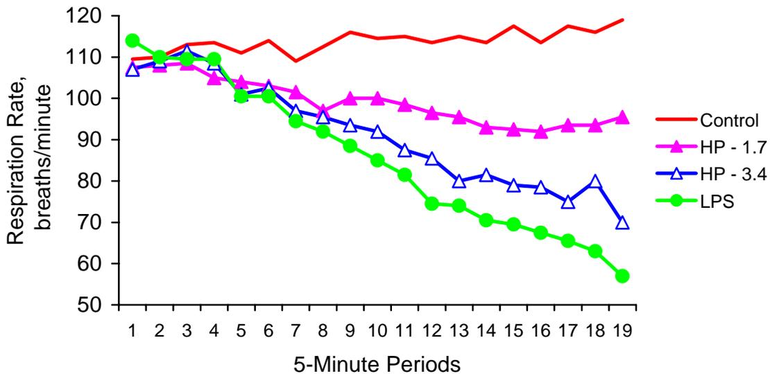
Control = no supplemental airflow or water treatment, HP-1.7 = 750 CFM airflow and 1.7 gallons/hour continuous high-pressure misting, HP-3.4 = 750 CFM airflow and 3.4 gallons/hour continuous high-pressure misting, and LPS = 750 CFM airflow and 4 gallons/hour of water via a low-pressure soaking system.
