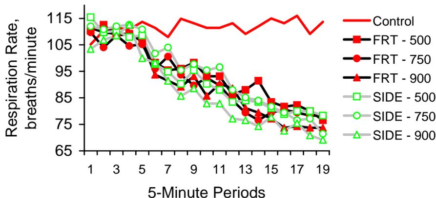
Control = no cooling system, FRT-500 = head to tail airflow at 500 CFM, FRT-750 = head to tail airflow at 750 CFM, FRT-900 = head to tail airflow at 900 CFM, SIDE-500 = right side airflow at 500 CFM, SIDE-750 = right side airflow at 750 CFM, and SIDE-900 = right side airflow at 900 CFM.
