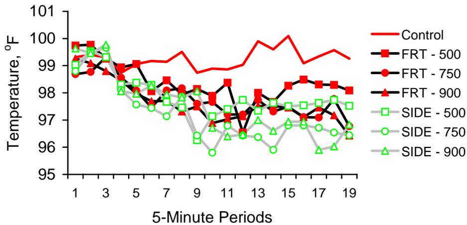
Control = no cooling system, FRT-500 = head to tail airflow at 500 CFM, FRT-750 = head to tail airflow at 750 CFM, FRT-900 = head to tail airflow at 900 CFM, SIDE-500 = right side airflow at 500 CFM, SIDE-750 = right side airflow at 750 CFM, and SIDE-900 = right side airflow at 900 CFM.
