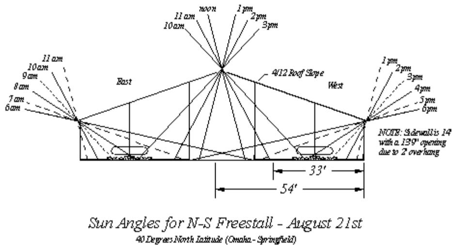
Figure 1. Sun Angles for a 4-Row Freestall Building Orientated North-South.
