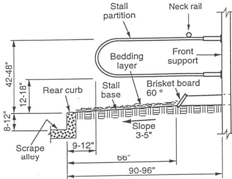
**Figure 1. Freestall Components and Dimensions.**
