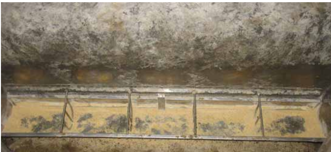
Figure 9. Conventional dry feeder at setting 8 with a 0.83- to 1.12-in. opening and \approx 57% pan coverage.
