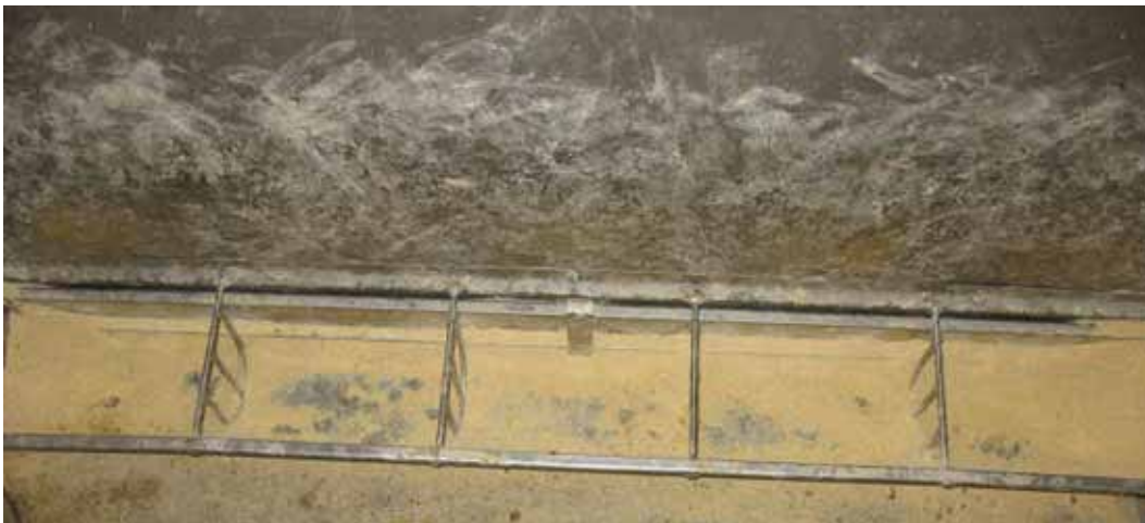
Figure 6. Conventional dry feeder at setting 10 with a 1.09- to 1.35-in. opening and \approx 79\% pan coverage.
