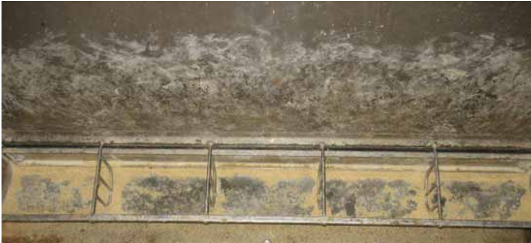
Figure 5. Conventional dry feeder at setting 8 with a 0.80- to 1.07-in. opening and \approx 21\% pan coverage.
