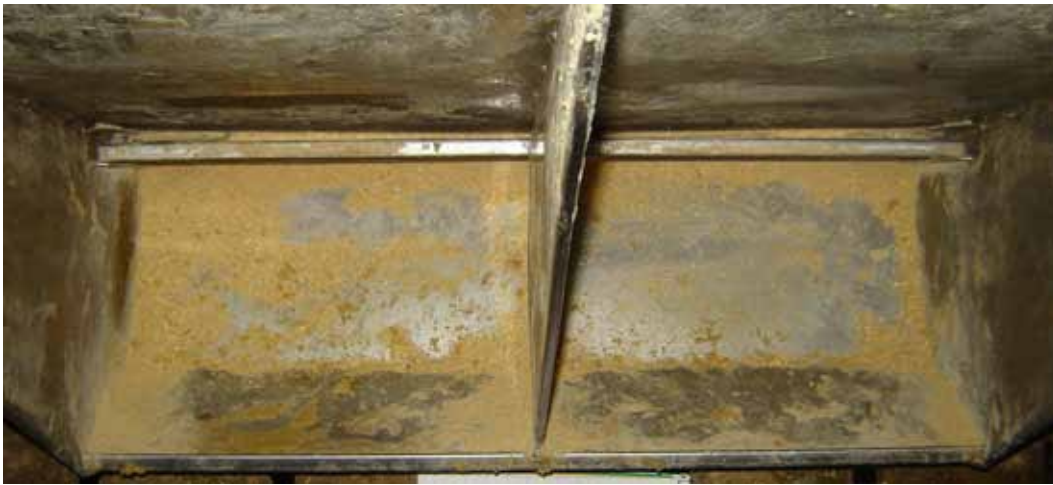
Figure 1. Narrow feeder adjustment (minimum feeder gap was 0.5 in. with a maximum gap of 0.75 in.) averaged 27% feeder pan coverage.
