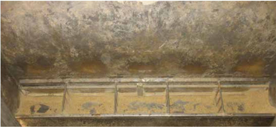
Figure 5. Conventional dry feeder at setting 8 with a 0.74- to 1.07-in. opening and \approx 67% pan coverage.
