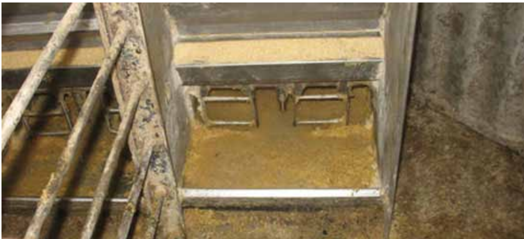
Figure 3. Wet-dry feeder at setting 14 with a 1.00-in. opening and \approx 83% pan coverage.
