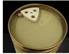
**Figure 2. Ball and Brush Resting of a Sieve.**
