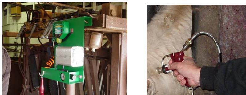
**Figure 1. Felton Pneumatic System and needle-free injector.**
