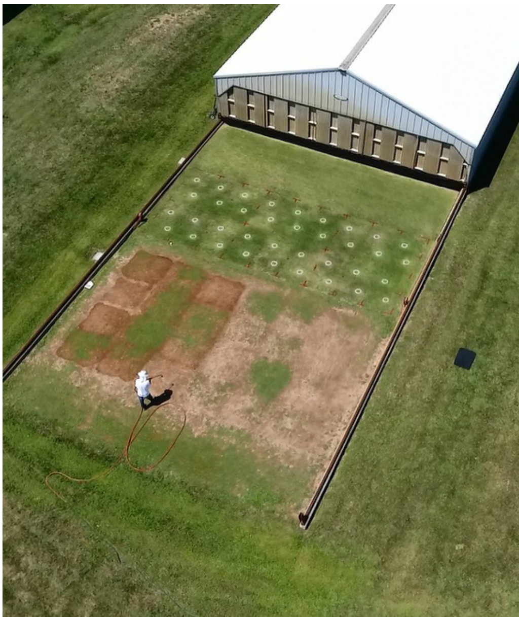
Figure 3. Deficit to well-watered irrigation treatment according to 15, 30, 50, 65, 80, and 100% reference evapotranspiration (ET) replacement. Irrigation was applied three times a week by hand with a wand attached to a meter.
