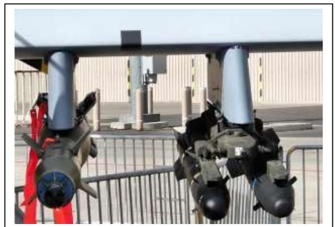
**Figure 11-4 Typical Reaper Load Out with the Hellfire Missiles on the right and a GBU-12 on the Left.** Twisted Sifter (2010). *The World’s Deadliest Drone: MQ-9 Reaper*. Retrieved From <https://twistedsifter.com/2010/05/worlds-deadliest-drone-mq-9-reaper/>
