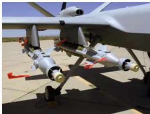
**Figure 11-9 Mq-9 Reaper With Gbu-38 Jdams Loaded.** Clark, C. (2017). Air Force drops first GPS bomb from Reaper: GBU-38 JDAM. Breaking defense. Retrieved from <https://breakingdefense.com/2017/05/air-force-drops-first-gps-bomb-from-reaper-gbu-38-jdam/>
