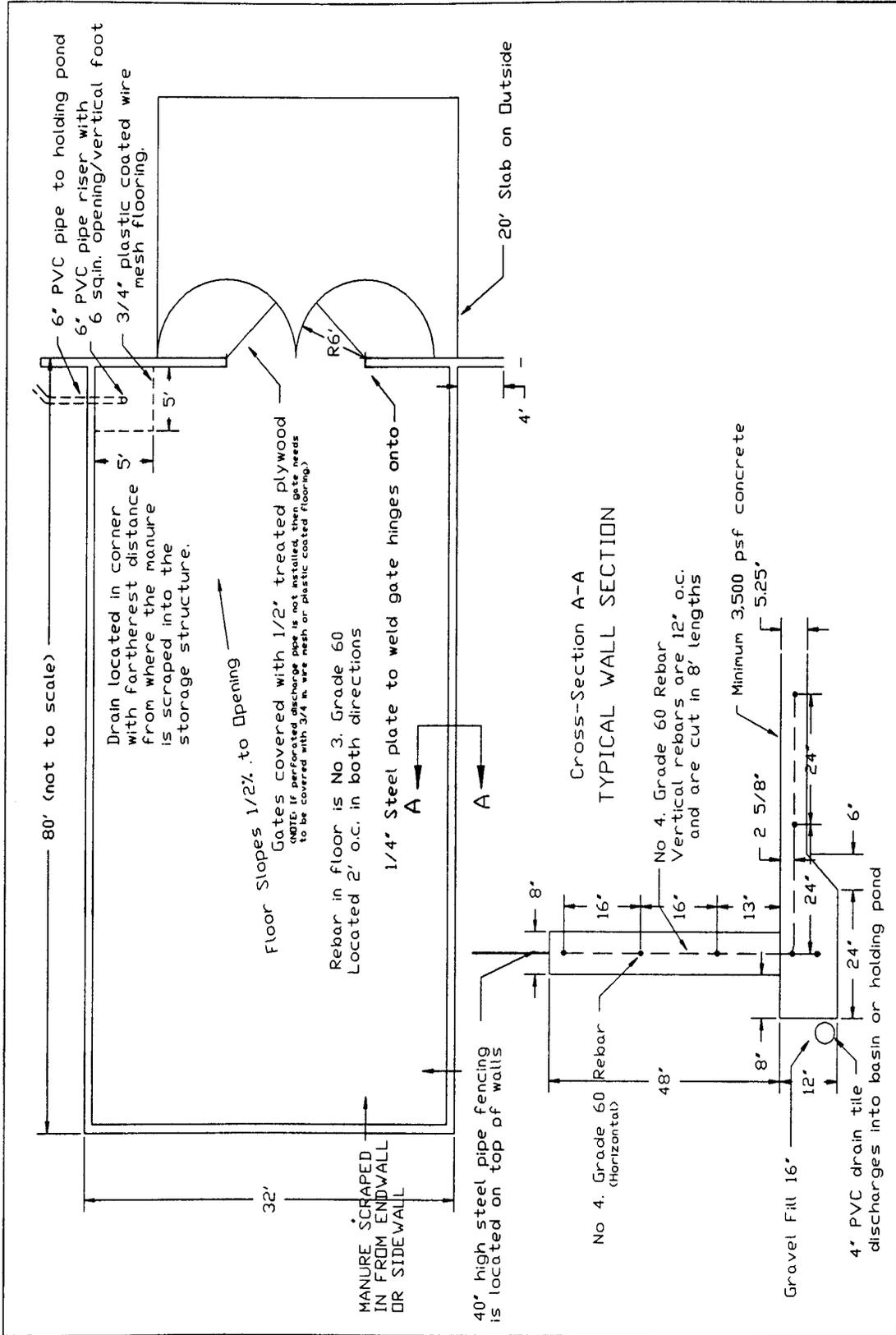
Figure 2. Concrete Level Bottom and Concrete Sidewall Structure
